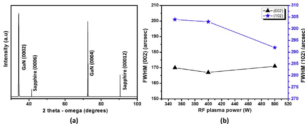
Fig. 1. (a) The 2-theta–omega scan of GaN film grown by rf-MBE at a plasma power of  $500$  W; (b) Plots of X-ray RC along (002) ( $\blacktriangle$ ) and (102) ( $\star$ ) plane w. r.t. rf plasma power.
