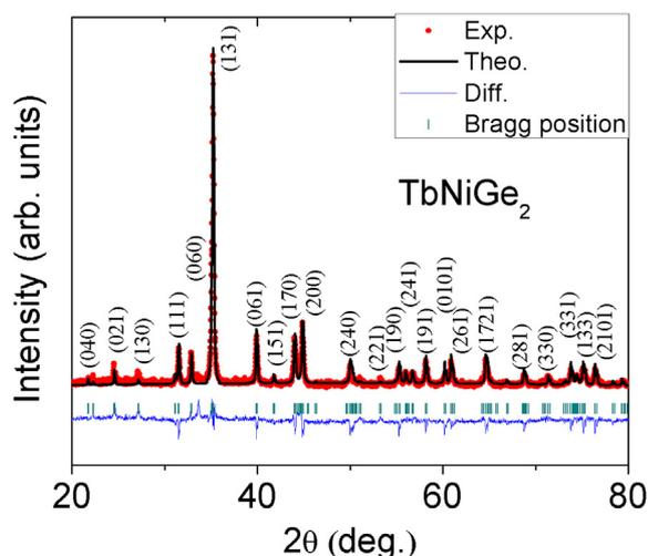
Fig. 1. The room temperature XRD pattern for TbNiGe $_2$ .
