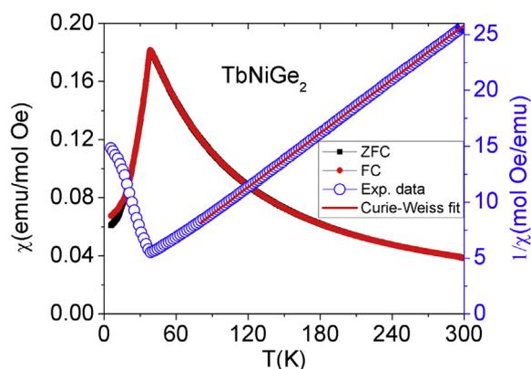
Fig. 2. Temperature dependence of magnetic susceptibility (left-hand scale) and inverse susceptibility along with the Curie–Weiss fit (right-hand scale) in 500 Oe for TbNiGe $_2$ .
