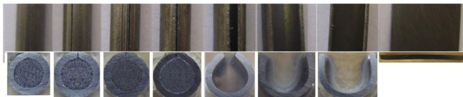
← Sequence of Manufacturing cored wire filler metal
