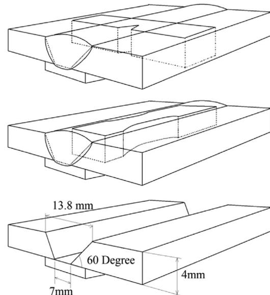
**Fig. 2.** Procedure of making specimens for tensile test and impact test after welding.
