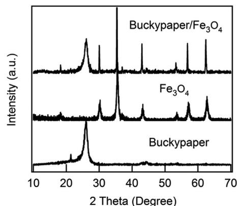
Fig. 2. X-ray diffraction patterns of the buckypaper,  $\text{Fe}_3\text{O}_4$  and  $\text{Fe}_3\text{O}_4$ /buckypaper composite samples.
