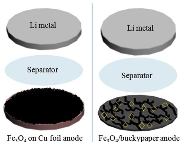
Fig. 1. A schematic illustration of a half-cell for testing of traditional  $\text{Fe}_3\text{O}_4$  on Cu foil anode and  $\text{Fe}_3\text{O}_4$ /buckypaper composite as anode.
