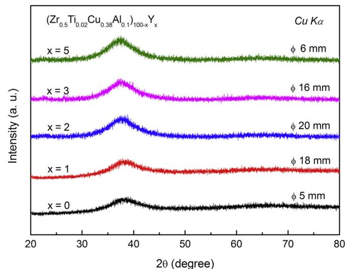
Fig. 1. XRD patterns of  $(Zr_{0.5}Ti_{0.02}Cu_{0.38}Al_{0.1})_{100-x}Y_x$  ( $x = 0, 1, 2, 3$  and 5 at.%) glassy rods with their critical diameters.
