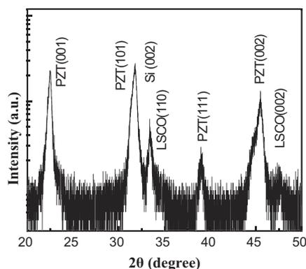
Fig. 1. XRD spectrum of the LSCO/PZT/LSCO/Nb-Ni/Si heterostructure.
