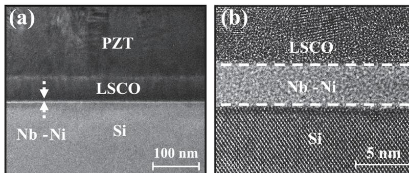
Fig. 2. (a) Cross-sectional image of the PZT/LSCO/Nb-Ni/Si of transmission electron microscopy (TEM); (b) high-resolution TEM cross-sectional image of the interfaces between Nb-Ni layer and its adjacent layer.
