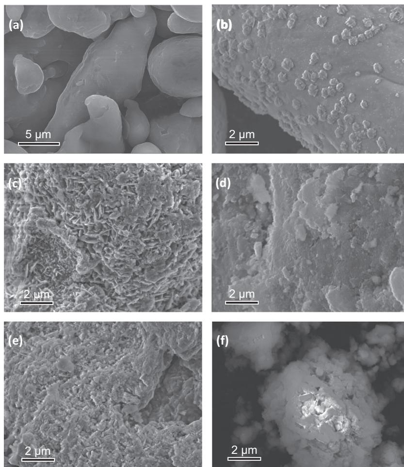
Fig. 1. SEM morphologies of Al powder (a) before and (b–f) after nitridation by different crafts, where (b) nitridation at 580 °C for 60 min, (c–f) nitridation at 600 °C for 30, 40, 60 and 120 min, respectively.
