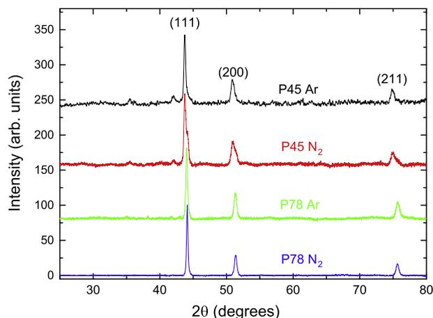
Fig. 1. XRD data from P45 and P78 made in Ar or N<sub>2</sub>. The data are offset for clarity and normalized to the same (111) peak intensity.
