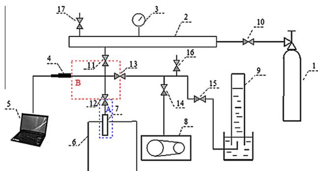
**Fig. 1.** Schematic representation of Sievert's apparatus for hydrogen adsorption.
