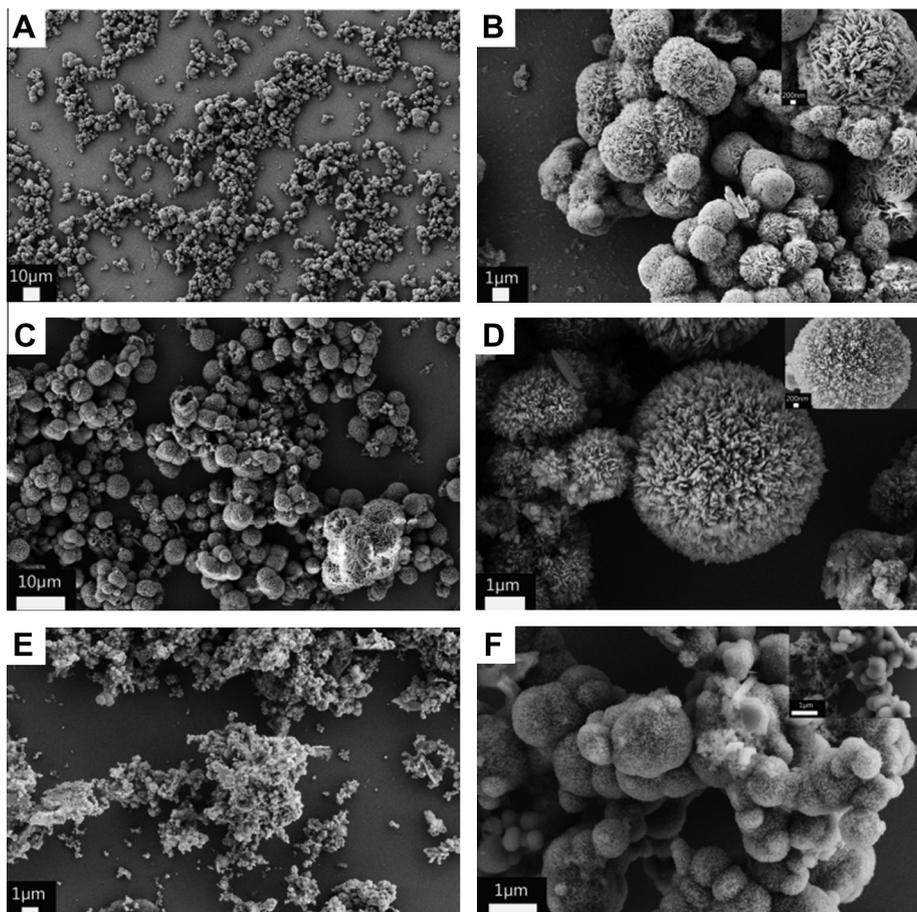
**Fig. 2.** SEM images of Mn-CPM, Co-CPM, and Zn-CPM. Low-magnification (A) and high-magnification (B) images of Mn-CPM (inset is a local magnification); low-magnification (C) and high-magnification (D) images of Co-CPM (inset is a local magnification); Low-magnification (E) and high-magnification (F) images of Zn-CPM (inset is a local magnification).
