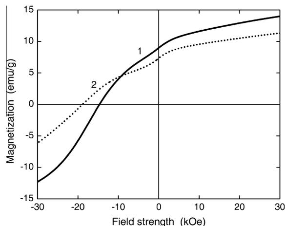
Fig. 3. Room-temperature demagnetization curves of as-synthesized samples: 1 – Nd-Fe-B, 2 –  $(\text{Nd}_{0.75}\text{Dy}_{0.25})\text{-Fe-B}$ . The curves are not corrected for self-demagnetization.
