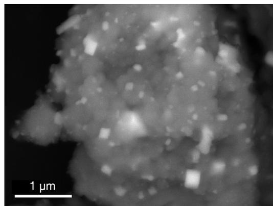
Fig. 2. Backscattered electrons SEM micrograph of as-synthesized  $(\text{Nd}_{0.75}\text{Dy}_{0.25})\text{-Fe-B}$  sample: bright  $\text{R}_2\text{Fe}_{14}\text{B}$  and R-rich particles are embedded in CaO/Ca matrix.
