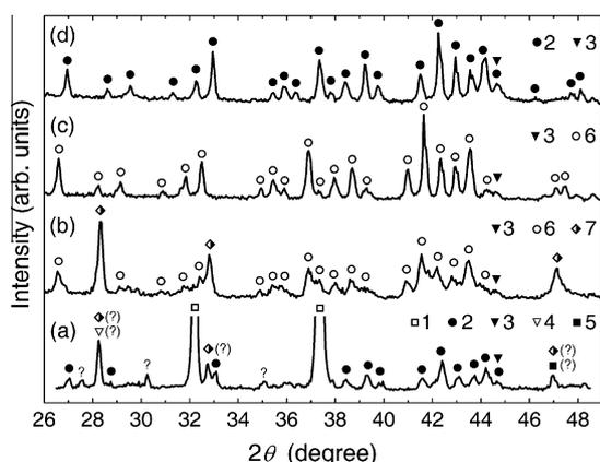
Fig. 1. XRD spectra of Nd-Fe-B sample (a) as-synthesized, (b) washed without acetic acid, (c) washed with acetic acid, (d) washed with acetic acid and annealed in vacuum at 400 °C. Identified structures: 1 – CaO, 2 –  $\text{Nd}_2\text{Fe}_{14}\text{B}$ , 3 – Fe, 4 – Ca, 5 –  $\text{Ca}(\text{OH})_2$ , 6 –  $\text{Nd}_2\text{Fe}_{14}\text{BH}_x$ , 7 –  $\text{Nd}_2\text{H}_5$ .
