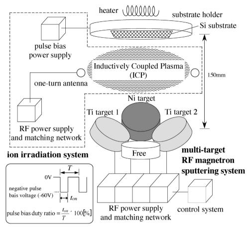
Fig. 1. Schematic illustration of a multi-target RF magnetron sputtering deposition system and ion irradiation system.
