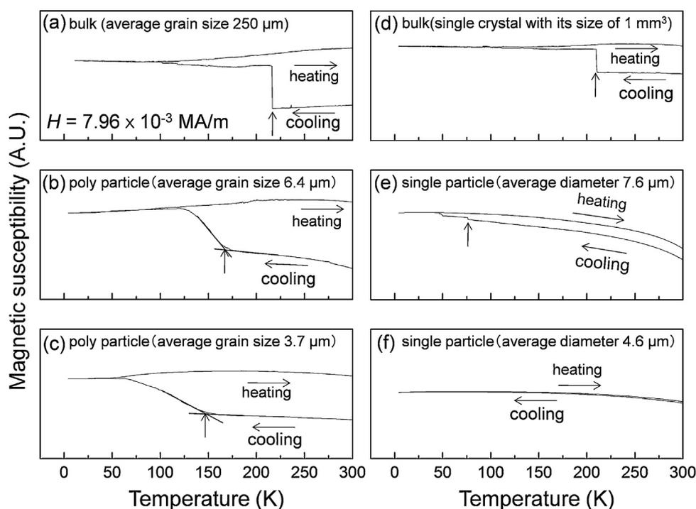
**Fig. 2.** Temperature dependence of magnetic susceptibility for each specimen in an Fe–30.5 at.%Ni alloy. Left figures are the results of poly crystalline particles and right figures are those of single crystalline particles.
