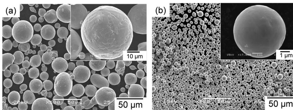
**Fig. 1.** Micrographs of particles in an Fe–30.5 at.%Ni alloy obtained by SEM observation. (a) and (b) are results of poly crystalline particle with its size of 25  $\mu\text{m}$  (average grain size is 6.7  $\mu\text{m}$ ) and that of single crystalline particle with its size of 7.6  $\mu\text{m}$ , respectively. The insets are magnified photos of (a) and (b).
