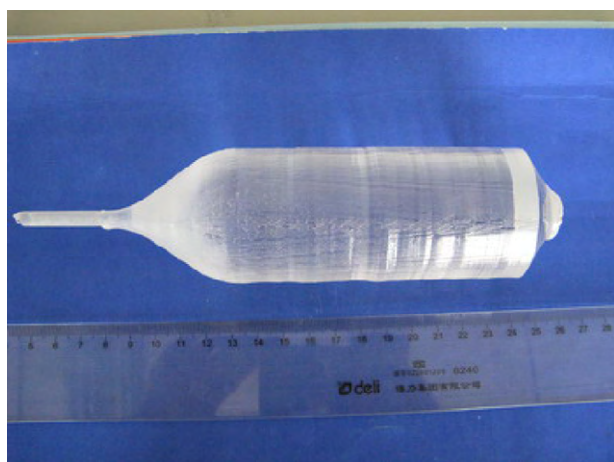
Fig. 1. The picture of pure YAP crystal with size of \varnothing 50 \text{ mm} \times 120 \text{ mm} .
