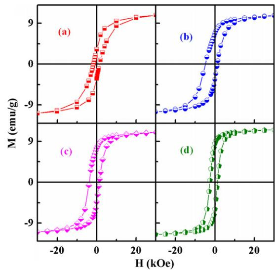
**Fig. 3.** Hysteresis loops measured at 10 K after field cooling at 10 kOe of a sample (b) milled for 3 h, and then annealed at (c) 573 K, and (d) 673 K; (a) hysteresis loop at 10 K measured after zero-field cooling of the sample milled for 3 h.
