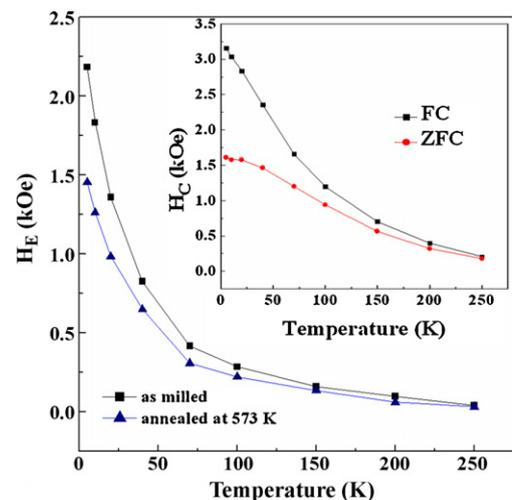
**Fig. 4.** Temperature dependence of  $H_E$  of powders, milled for 3 h and then annealed at 573 K for 30 min, after field cooling in 10 kOe from 295 K. Inset: coercivity of as-milled Ni/NiO powders vs temperature ( $T$ ) measured after ZFC and FC.
