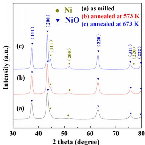
**Fig. 2.** X-ray diffraction patterns of samples (a) milled for 3 h, and then annealed at (b) 573 K, (c) 673 K for 30 min in a vacuum furnace.
