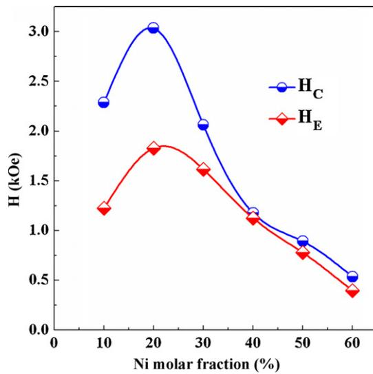
**Fig. 1.** Dependence of the loop shift ( $H_E$ ) and the coercivity ( $H_C$ ) on the FM (Ni) molar fraction for as-milled Ni/NiO powders, measured at 10 K.
