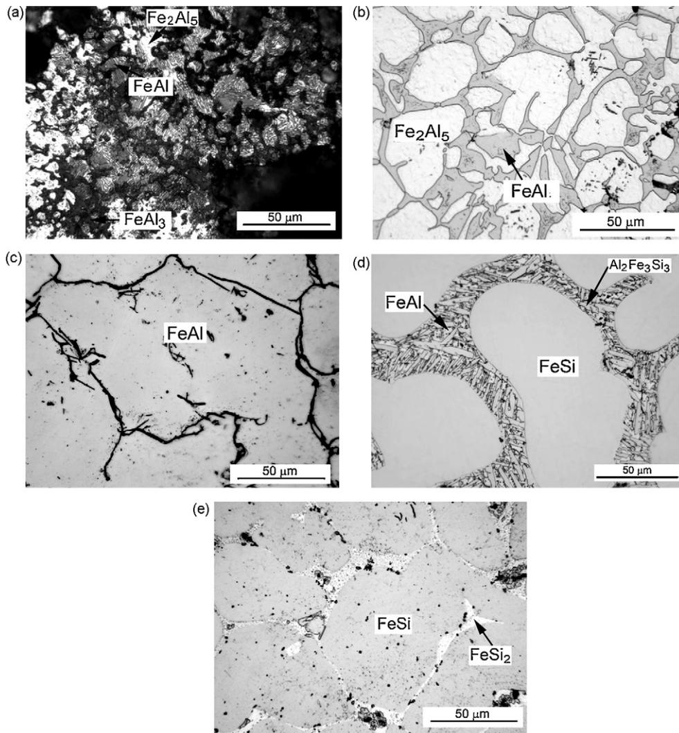
**Fig. 1.** Microstructure of Fe–Al, Fe–Al–Si and Fe–Si alloys produced by reactive sintering (1100 °C, 30 min): (a) FeAl40, (b) FeAl35Si5, (c) FeAl30Si10, (d) FeAl20Si20 and (e) FeSi40.
