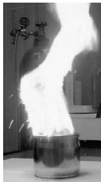
Fig. 1. Typical reaction followed by flame in the mixed powder after opening the vial lid (sample 1–8).
