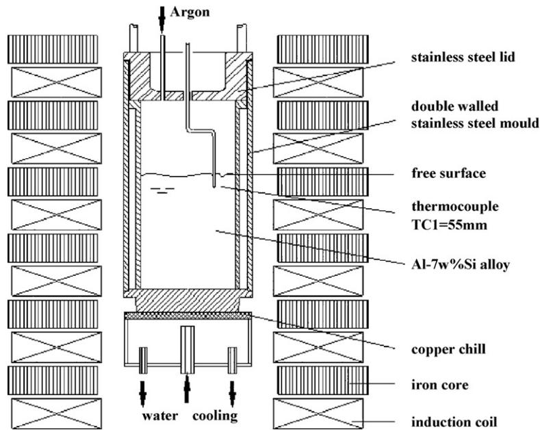
Fig. 1. Schematic view of the experimental set-up.
