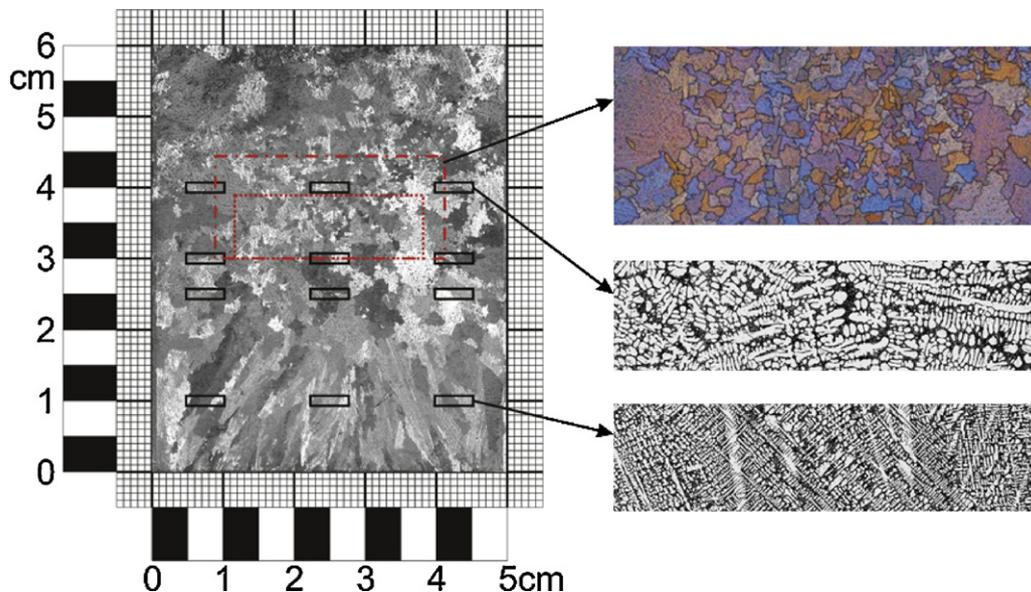
Fig. 2. Longitudinal section of a solidified sample showing the locations of inspection windows for quantitative examinations of the grain morphology.
