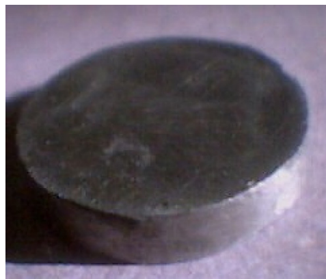
Fig. 2. Photograph of thermal explosion-pressing specimen.
