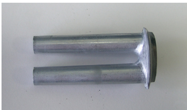
Fig. 1. Part produced from A365 alloy via thixoforming.
