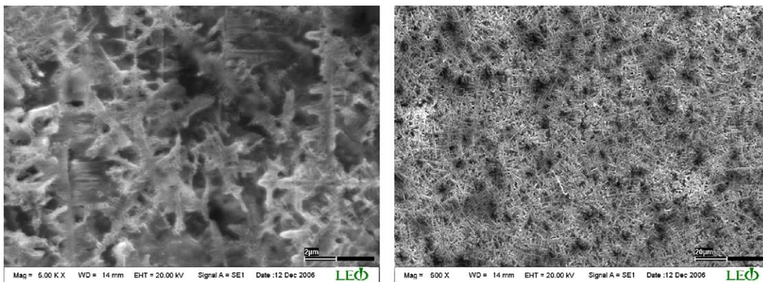
Fig. 2. SEM photographs of the  $\text{La}_{0.67}\text{Ba}_{0.33}\text{MnO}_3$  film sample.
