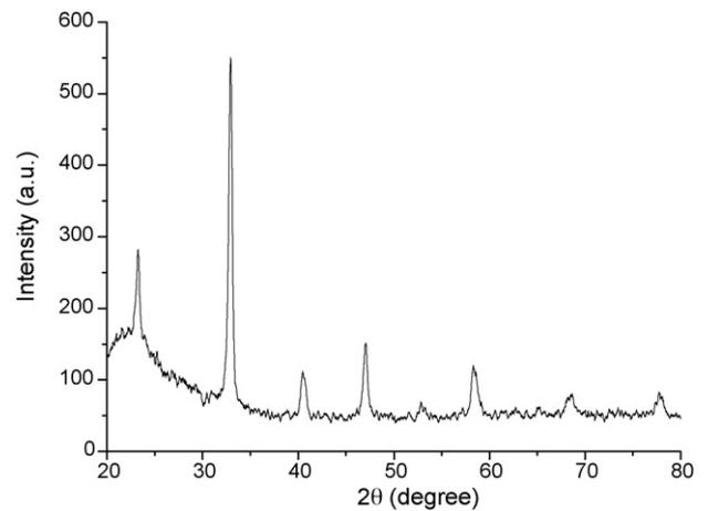
Fig. 1. X-ray diffraction patterns of the  $\text{La}_{0.67}\text{Ba}_{0.33}\text{MnO}_3$  film produced on quartz substrate.
