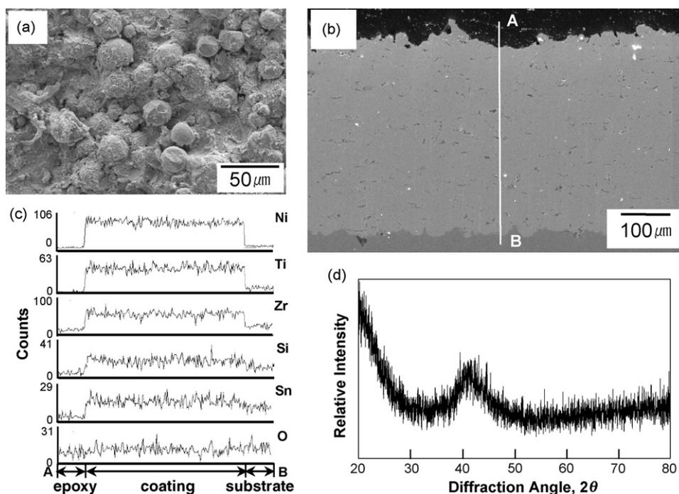
Fig. 1. Bulk amorphous  $\text{Ni}_{57}\text{Ti}_{18}\text{Zr}_{20}\text{Si}_3\text{Sn}_2$  coating. (a) SEM top view, (b) SEM cross-sectional image, (c) EDS line profiles and (d) XRD pattern.
