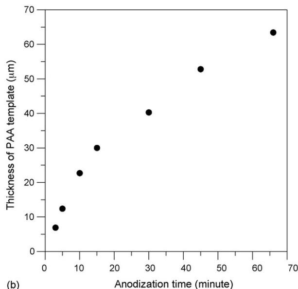
Fig. 2. (a) SEM top-view image of PAA template. (b) PAA thickness plotted as a function of anodization time.
