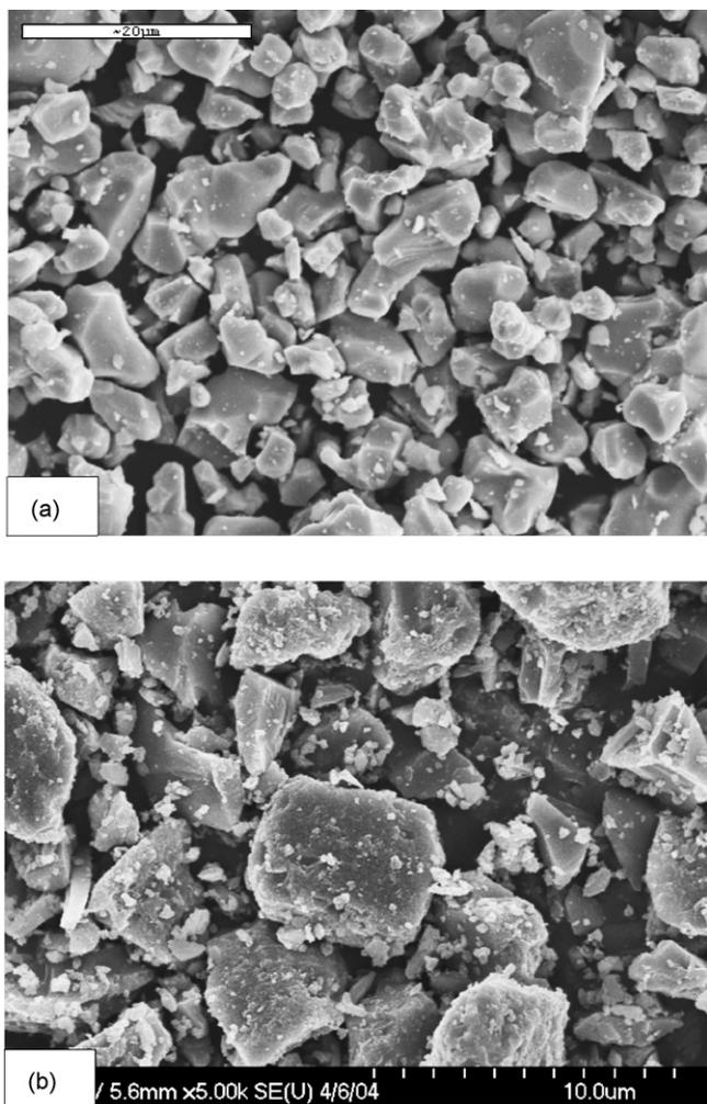
Fig. 1. Scanning electron microscope images of raw materials: (a) niobium carbide and (b) silicon powder.
