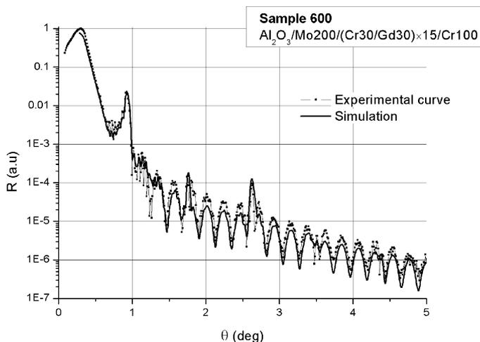
Fig. 1. Experimental and simulation reflectivity curves for sample  $\text{Al}_2\text{O}_3/\text{Mo}200/(\text{Cr}30/\text{Gd}30) \times 15/\text{Cr}100$  grown at room temperature.
