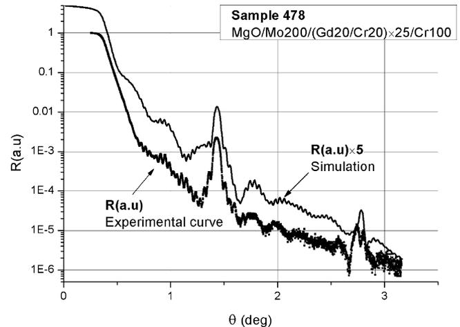
Fig. 2. Experimental and simulation reflectivity curves for  $\text{MgO}/\text{Mo}200/(\text{Cr}20/\text{Gd}20) \times 25/\text{Cr}100$  multilayer grown at room temperature. The intensity of simulated curve was multiplied by a factor of 5 in order to easily distinguish both curves.
