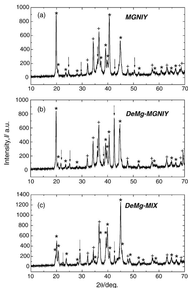
Fig. 1. X-ray diffraction patterns of the prepared materials MGNIY, DeMg–MGNIY and DeMg–MIX. “\*” and “+” mean Mg<sub>2</sub>Ni and Mg peaks, respectively. Arrows indicate unidentified peaks.
