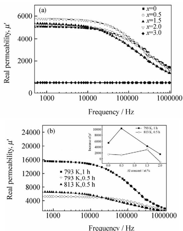
**Fig. 1.** Dependences of real permeability spectra on Al content (a) and annealing condition (b): (a) annealed at 793 K for 0.5 h; (b)  $x = 0.5$ , annealed at different conditions. The inset gives the increase of  $\mu'$  for  $\text{Fe}_{73.5}\text{Si}_{13.5}\text{B}_9\text{Cu}_1\text{Nb}_{3-x}\text{Al}_x$  ( $x = 0, 0.5, 1.5, \text{ and } 2.0$ ) ribbons annealed at 793 K for 1 h and at 813 K for 0.5 h compared to that annealed at 793 K for 0.5 h (measured at 0.265 A/m and 1 kHz).
