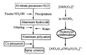
Fig. 1. Schematic diagram displaying the procedure for the preparation of the spray solution containing aluminum polycations.
