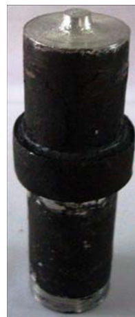
Fig. 2 Fabricated friction stir processing tool
