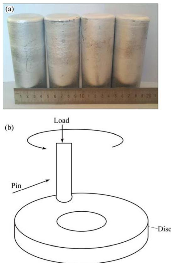
**Fig. 1** Ingots of matrix alloy and composites (a) and schematic diagram of pin-on-disc wear test (b)
