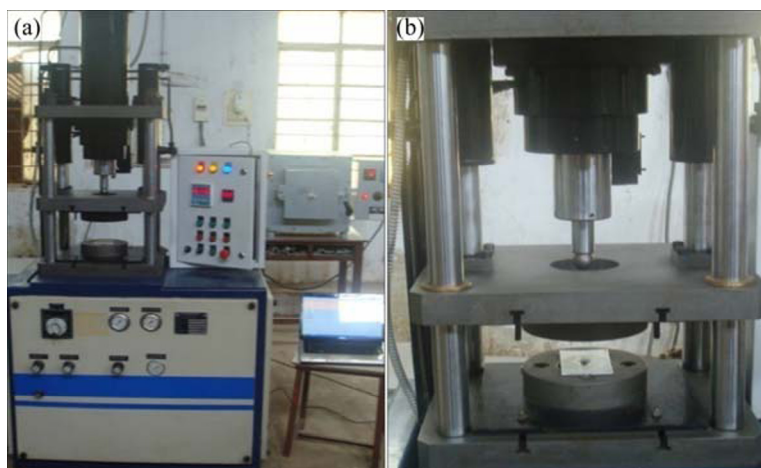
Fig. 2 Hydraulic press (a) and punch, dies and welded blank (b)
