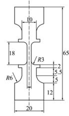
Fig. 1 Creep testing sample (unit: mm)
