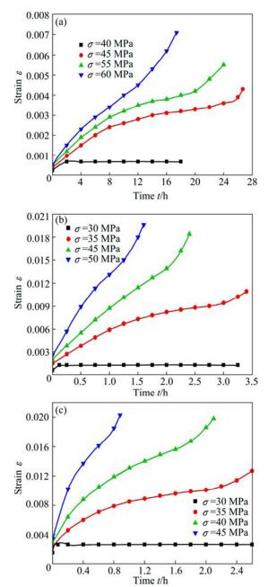
**Fig. 2** Creep curves of AZ91 magnesium alloy under different stresses and temperatures: (a) 473 K; (b) 523 K; (c) 573 K
