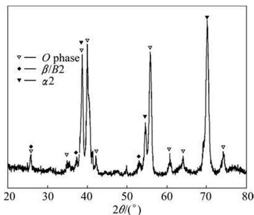
**Fig. 2** X-ray diffraction pattern of as-soluted Ti–22Al–26Nb–1Zr alloy
