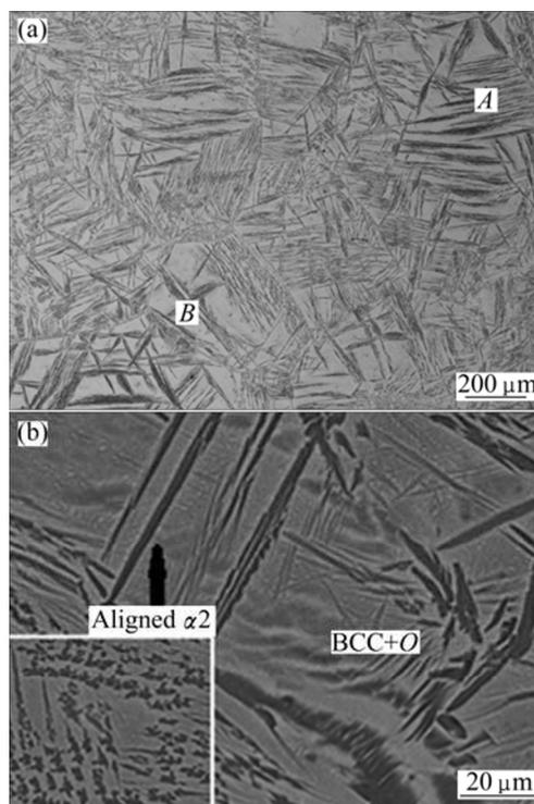
**Fig. 1** Optical (a) and back scattered SEM (b) images of Ti–22Al–26Nb–1Zr alloy after heating in the  $B2$  phase field for 1 h followed by furnace cooling
