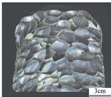
Fig. 1 Typical vertical section of aluminum foams produced at 680 °C
