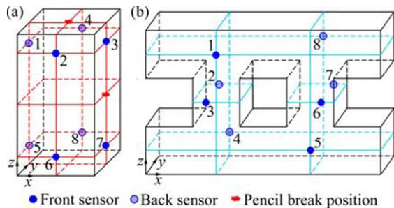
Fig. 1 Configuration of AE sensors: (a) Pencil break specimen; (b) Pillar specimen
