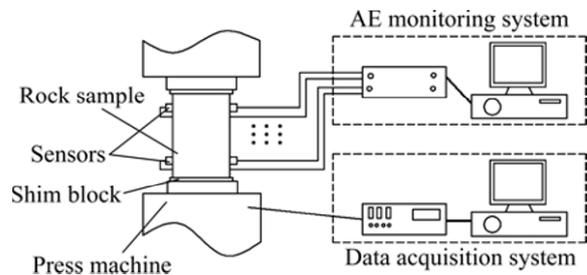
Fig. 2 Schematic diagram of AE and loading system
