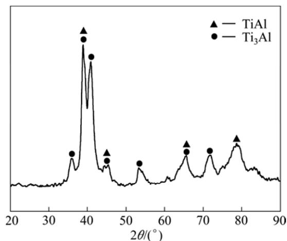
**Fig. 2** XRD pattern of Ti–45Al–5.5(Cr,Nb,B,Ta) powder after high energy mechanical milling
