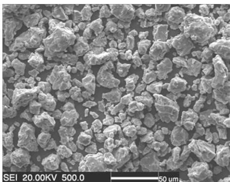
**Fig. 1** SEM image of high energy mechanically milled Ti–45Al–5.5(Cr,Nb,B,Ta) powder
