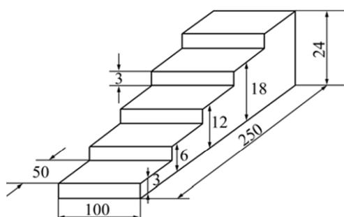
Fig. 1 Stepped pattern designed for experiments (Unit: mm)
