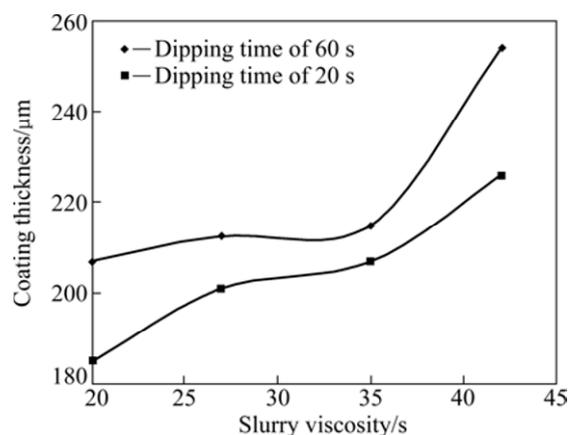
Fig. 2 Effect of slurry viscosity and dipping time on coating thickness
