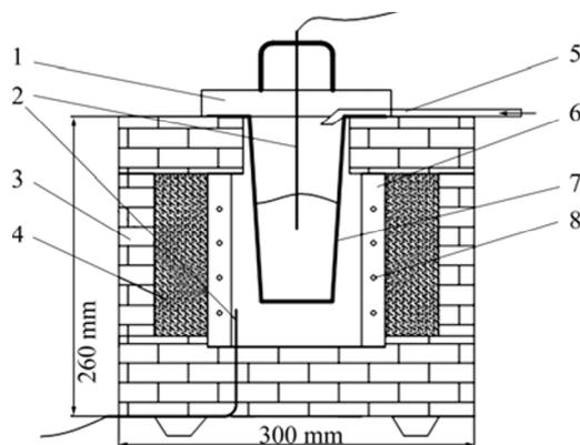
**Fig. 1** Schematic diagram of melting device of magnesium alloy: 1—Furnace lid; 2—Heat electric couple; 3—Refractory brick; 4—Mineral flax; 5—Gas-guide tube; 6—Internal furnace; 7—Crucible; 8—Resistance wire
