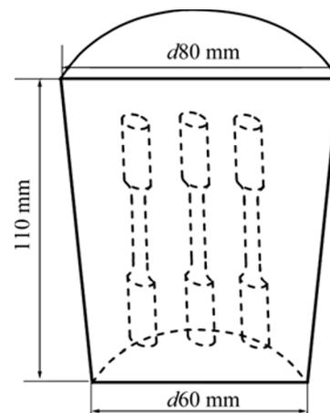
**Fig. 2** Schematic diagram of casting and sampling location
