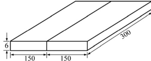
Fig. 1 Square butt joint configuration (Unit: mm)
