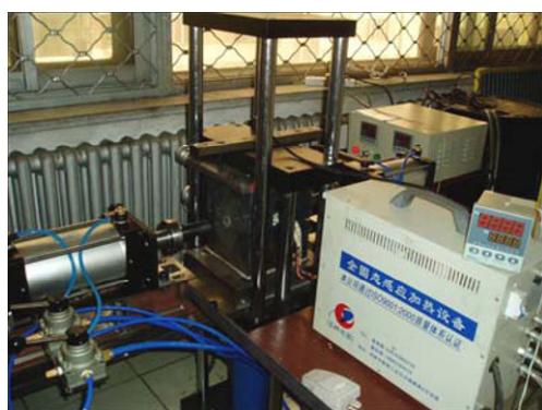
Fig. 1 Experimental setup for hot metal gas forming
