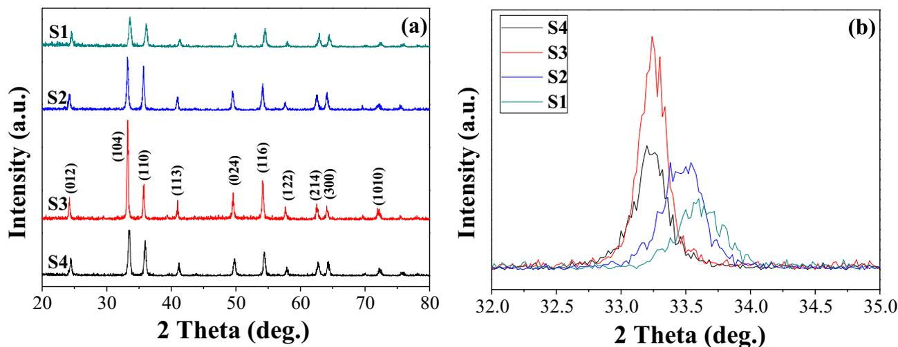
Fig. 1. XRD patterns of S1 (20 vol% ethanol–water mixed solvent), S2 (50 vol% ethanol–water mixed solvent), S3 (80 vol% ethanol–water mixed solvent) and S4 (90 vol% ethanol–water mixed solvent).
