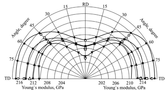
**Fig. 1.** The Young's modulus anisotropy in the DP600 steel sheet: ● – after annealing at 220 °C, ■ – subsequent tensile deformation of 3%, ▲ – 6%, ▼ – 10%, ○, △, ▽ – control measurements of Young's modulus.
