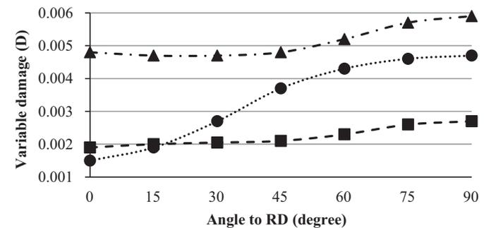
**Fig. 2.** Damage coefficient anisotropy of DP600 steel sheets after long time annealing and subsequent tensile deformation up to: ● – 3%, ■ – 6% and ▲ – 10% deformation.
