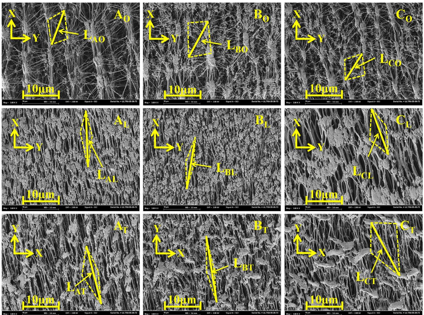
Fig. 1. SEM images of the released and stretched PTFE microporous materials. A<sub>0</sub>, B<sub>0</sub> and C<sub>0</sub> refers to the released samples with average pore size of 0.22 μm, 0.17 μm and 0.2 μm, respectively. A<sub>L</sub>, B<sub>L</sub> and C<sub>L</sub> refer to the stretched samples after longitudinal elastic deformation. A<sub>T</sub>, B<sub>T</sub> and C<sub>T</sub> refer to the stretched samples after transverse elastic deformation.
