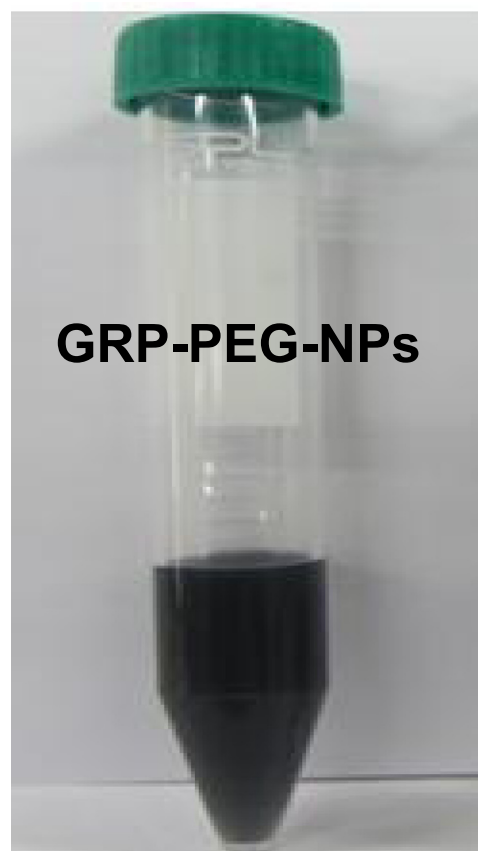
Fig. 2. Photographic image of the sample GRP-PEG-NPs, showing the stable dispersion.
