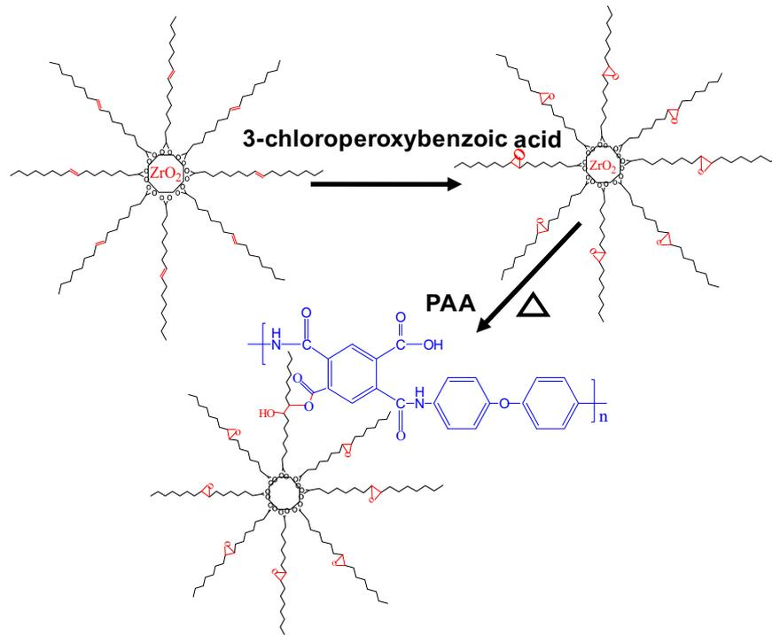
Fig. 1. Mechanism of modified  $ZrO_2$  nanocrystals and the formation of polyimide/ $ZrO_2$ -nanocrystals hybrid thin films.
