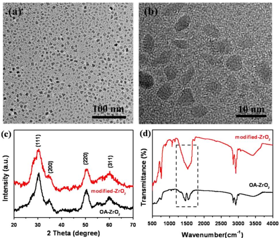
Fig. 2. LR-TEM (a) and HR-TEM (b) images of  $ZrO_2$  nanocrystals; XRD patterns (c) and FT-IR spectra (d) of OA-capped  $ZrO_2$  nanocrystals and modified  $ZrO_2$  nanocrystals. (For interpretation of the references to color in this figure legend, the reader is referred to the web version of this article.)
