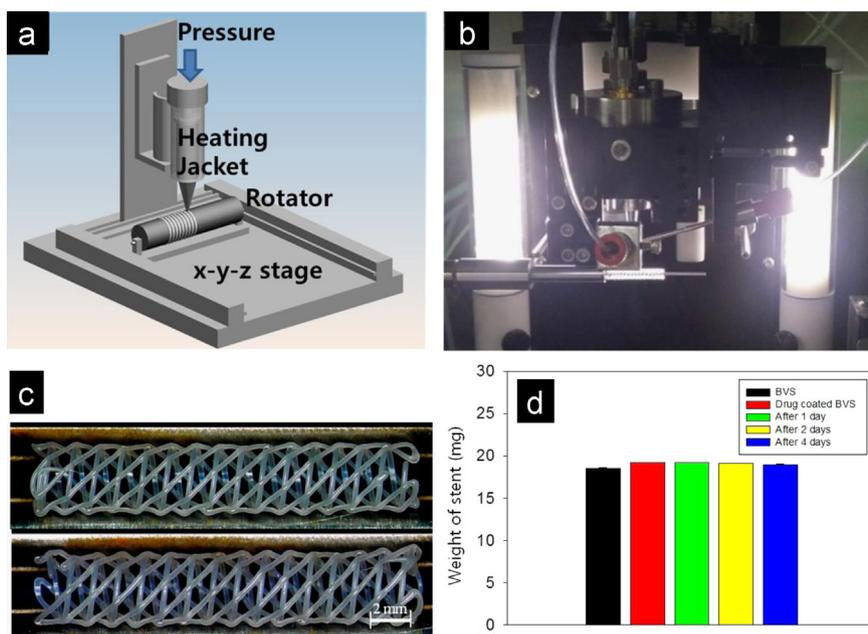
Fig. 1. Schematic design of a 3D printing system (a), an ultrasonic-spray coating system (b), an optical microscope image (c), and a weight changes (d).
