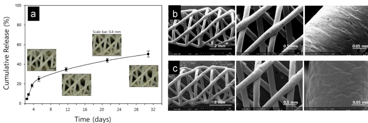
Fig. 2. Cumulative release of sirolimus (a) and SEM image of BVS (b) and sirolimus coated BVS (c) after zero day.
