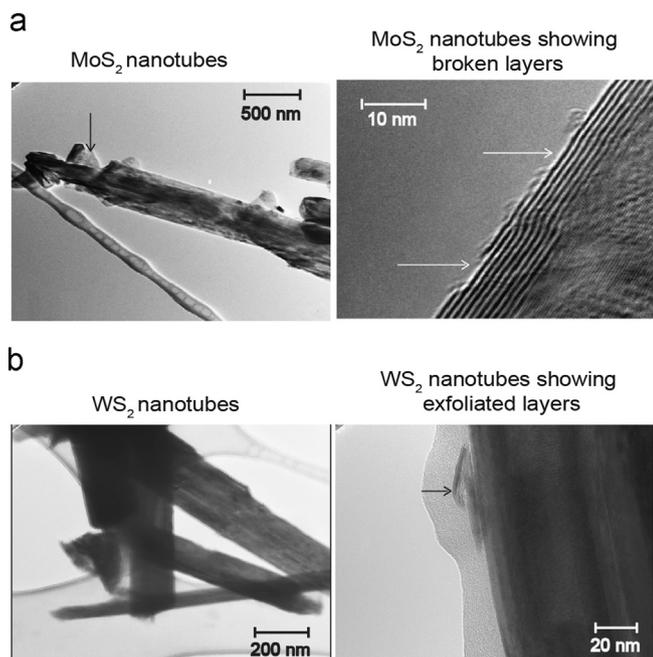
Fig. 1. TEM images of (a) MoS<sub>2</sub> nanotube with a broken edge (Top), magnified image showing broken surface layers (Right), (b) agglomerated WS<sub>2</sub> nanotubes (Left), a magnified image with an arrow pointing to exfoliated layers (Right) and a magnified image of a nanotube showing ordered layers (Maharaj and Bhushan, 2014).
