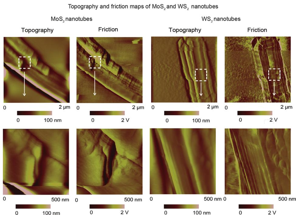
Fig. 2. Examples of topography and friction maps of MoS<sub>2</sub> (Left) and WS<sub>2</sub> nanotubes (Right) with arrows pointing to magnified images of the areas highlighted by dashed squares.
