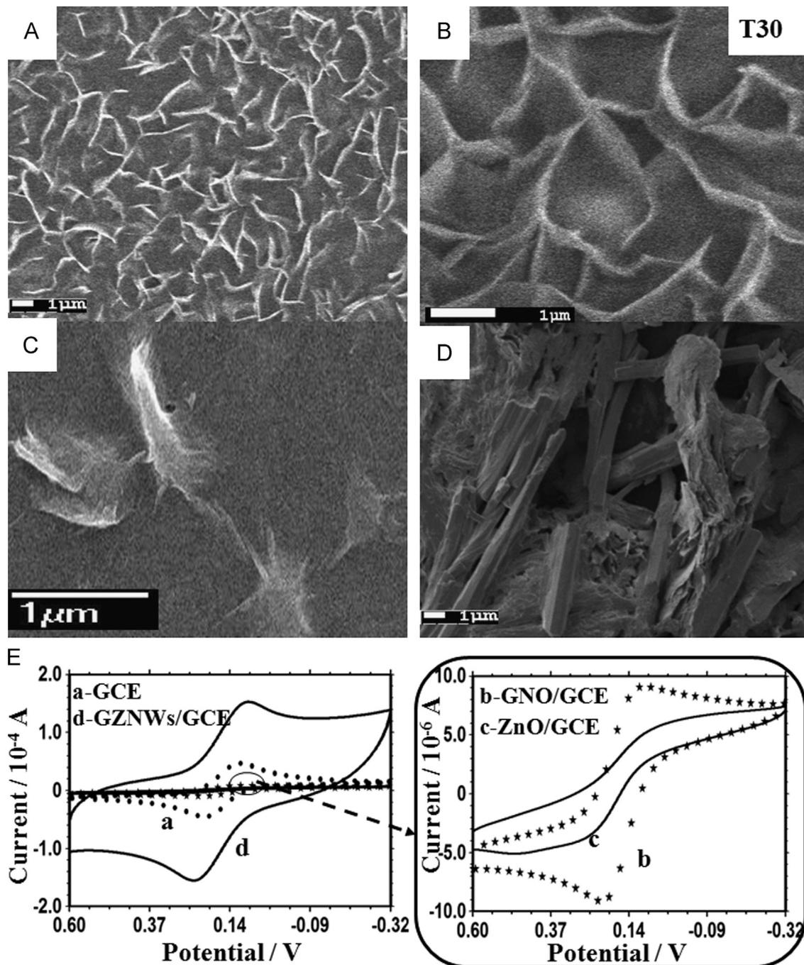
**Fig. 1.** SEM micrographs of the GZNWs-20 min ((A) top view), GZNWs-20 min ((B) tilted with an inclination angle of  $30^\circ$ ), (C) GNO, (D) ZnO without GNO support, and (E) cyclic voltammograms of 2 mmol/L  $[\text{Fe}(\text{CN})_6]^{3-/4-}$  (1:1) at bare GCE (a), GNO/GCE (b), ZnO/GCE (c) and GZNWs/GCE (d).
