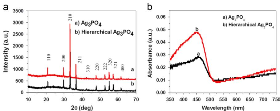
Fig. 2. XRD pattern (a) and UV–vis DRS of the as-synthesized conventional Ag<sub>3</sub>PO<sub>4</sub> and hierarchical Ag<sub>3</sub>PO<sub>4</sub> photocatalysts.
