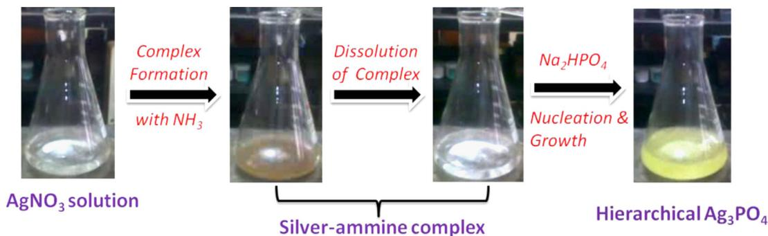
Fig. 1. Schematic diagram with photographs for synthesis of hierarchical Ag<sub>3</sub>PO<sub>4</sub> microcrystals.
