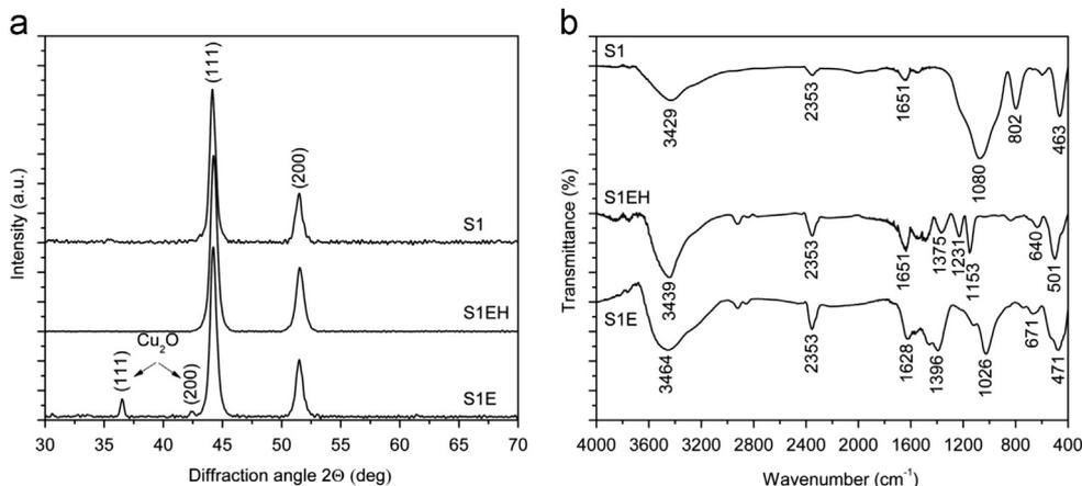
Fig. 1. X-ray diffraction patterns (a) and FTIR spectra (b) of as-prepared sample in SiO<sub>2</sub> matrix (S1), etched S1 sample in etching solution, with (S1EH) and without hydrazine hydrate (S1E).
