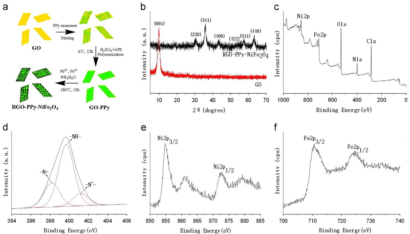
Fig. 1. Schematic illustration (a), XRD patterns of GO and RGO-PPy-NiFe<sub>2</sub>O<sub>4</sub> (b), XPS spectrum (c), N 1s (d), Ni 2p (e) and Fe 2p (f) spectra of RGO-PPy-NiFe<sub>2</sub>O<sub>4</sub>.
